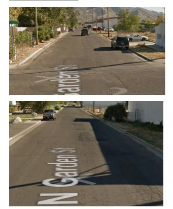
This section has asphalt widths from 26 feet to 30 feet. There are 3 hydrants in this section on either end and in the center.
