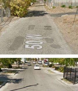
Fire recommends that asphalt widths adhere to 30 feet as stated in Tooele City Code 7-4-11. Recently passed State Legislation for residential roadways is currently set at 32 feet of asphalt. The asphalt on the North end of this section has been improved as opposed to the South end.
